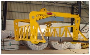
**Tripoid Grab** *Material:* 5.5M diameter forged rings, *Capacities:* Upto 10MT, *Temperature:* Upto 1200°C
